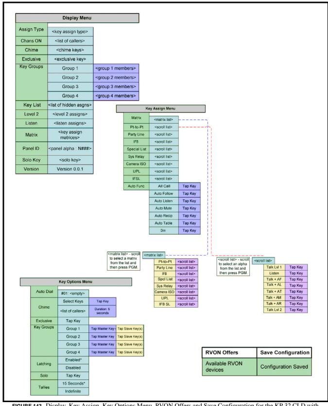
**FIGURE 143.** Display, Key Assign, Key Options Menu, RVON Offers and Save Configuration for the KP 32 CLD with GPI 32 CLD Option card installed. RVON Offers only displays if the keypanel is connected to an RVON device, otherwise the menu item is not available
